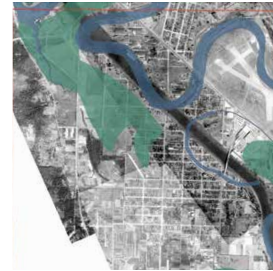
Historical channel of the Duwamish River overlaid on a aerial of South Park ca. 1940. Note that the river has been channelized by this point.
